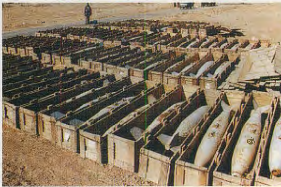
(left) UN weapons' inspectors in Iraq discovered thousands of bombs containing chemical weapons (such as these 250-kg bombs that originally held mustard gas). Many were found to be damaged and leaking in their storage areas. (below) America's 'Honest John' warhead held scores of bomblets filled with sarin nerve gas. They were designed to scatter these munitions near the intended target.
